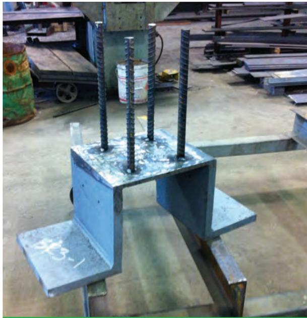
The column-to-column connector with saddles to carry glulam beams
