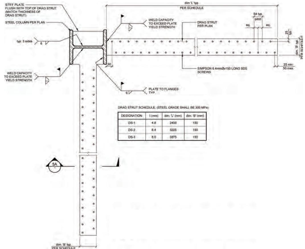
Typical Drag Strut Plan View
