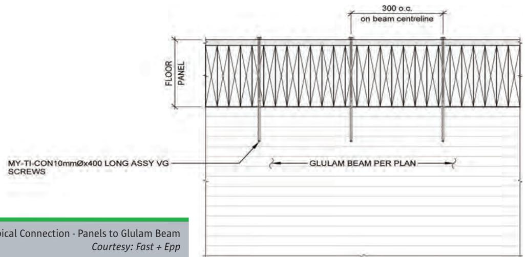
Solid Sawn Lumber Floor - Typical Connection - Panels to Glulam Beam
