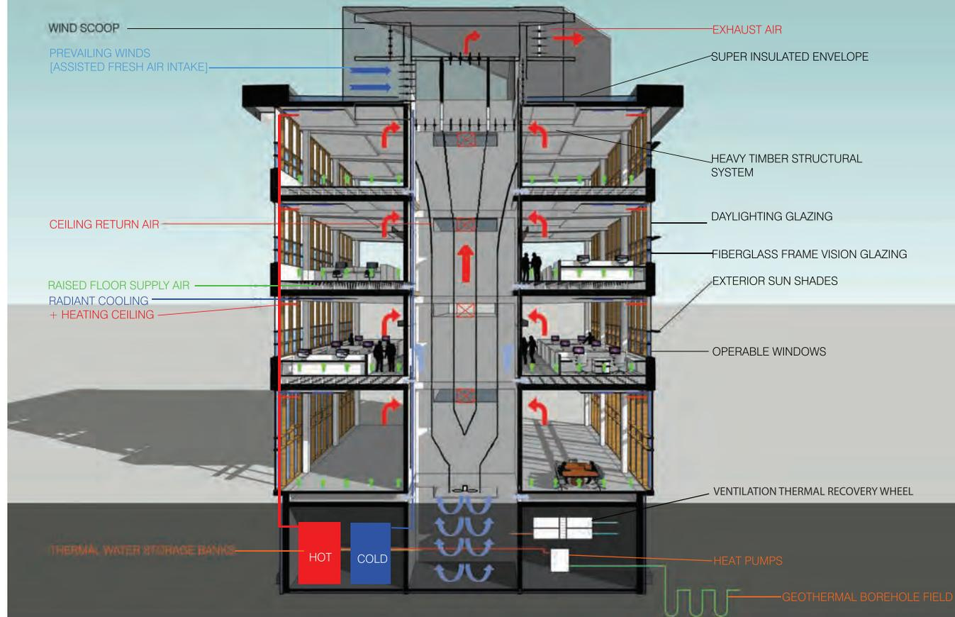
Natural Hybrid Ventilation / Thermal Recovery Systems and Environmental Features
